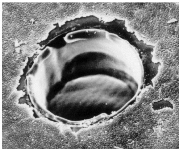
Fig. 2: Ideal ablation crater with 40 \mu\text{m} diameter. Abb. 2: Idealer Ablationskrater von 40 \mu\text{m} Durchmesser (Source / Quelle: Lambda Physics).
