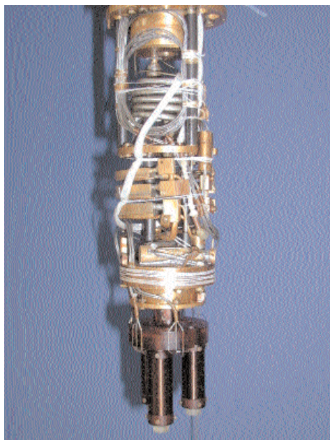
Fig. 1: Lower part of the dilution refrigerator showing the three experimental towers for SQUID inductive measurements.
