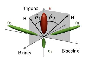
Fig. 3: The Fermi surface of bismuth consists of a hole pocket (red) and three electron pockets (green).  $\theta I \ (\theta 2)$  show angles between the magnetic field and the trigonal axis in the trigonal-binary (trigonal-bisectrix) rotating plane (taken from [12]).
