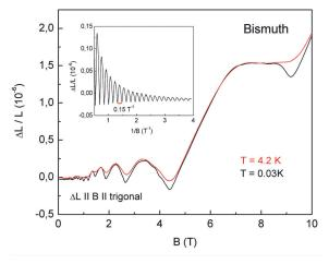
Fig. 4: Quantum oscillations of the magnetostriction for a field along trigonal at T = 0.03 and 4.2 K. Inset: Low-field oscillatory magnetostriction at 0.03 K, up to 2 T.
