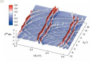
Fig. 5: Quantum oscillations observed in the 2<sup>nd</sup> derivative of the magnetostriction data, divided by  $B^2$ , with a tilted magnetic field (trigonal to bisectrix) up to 10 T at T = 30 mK.
