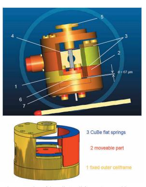
Fig. 1: Drawing of the cell. 1: cell frame, 2: moveable part, 3: CuBe flat springs, 4: sample, 5: adjustment screw, 6: upper capacitor plate, 7: lower capacitor plate.
