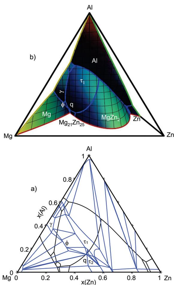
Fig. 1: Isothermal section of the Al-Mg-Zn system at 330 °C with liquidus curve projection (a); 3D view of the liquidus surface (b).
