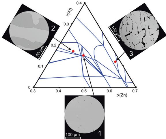
Fig. 4: Part of the isothermal section of the Al-Mg-Zn system at 330 °C in the vicinity of the  $\tau_2$  phase and micrographs (BSE) for alloys at various compositions proposed for single-phase  $\tau_2$ : 1)  $\text{Al}_{15}\text{Mg}_{43}\text{Zn}_{42}$ , 2)  $\text{Al}_{17}\text{Mg}_{46}\text{Zn}_{37}$ , 3)  $\text{Al}_{13}\text{Mg}_{32}\text{Zn}_{55}$ .
