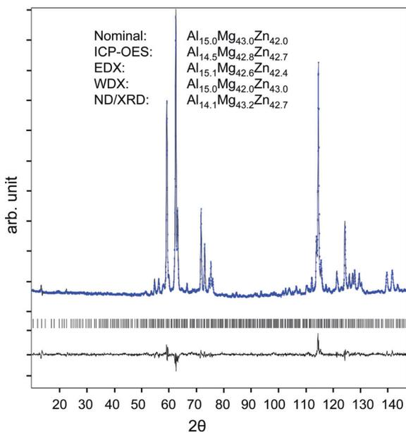
Fig. 5: Intensity versus  $2\theta$ -plots of the observed and calculated neutron pattern of  $\tau_2$  at  $\text{Al}_{15}\text{Mg}_{43}\text{Zn}_{42}$ ; X-ray and neutron data have been combined in the Rietveld refinement.
