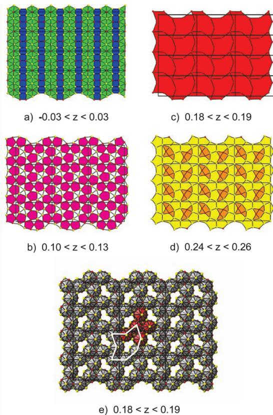
Fig. 3: The four different atom layer types in the crystal structure of the  $\Phi$  phase are shown as tilings: a) square-triangle tiling, b) pentagon-triangle tiling, c) boat tiling, d) pentagon-boat tiling, e) decoration of boat tiling by icosahedra; one cluster is shown in red colour.
