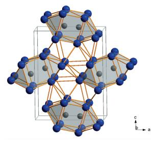
Fig. 1: Crystal structure of  $CoBi_3$ . The capped trigonal prisms of bismuth atoms (in blue) form chains along the *b* axis and contain the cobalt atoms (in gray).
