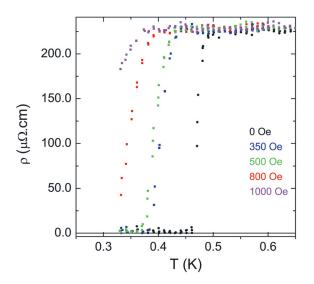
Fig. 2: Temperature dependence of the electrical resistivity of the polycrystalline CoBi<sub>3</sub> for different applied magnetic fields.
