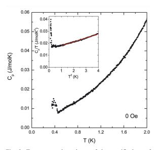
Fig. 3: Temperature dependence of the specific heat of polycrystalline CoBi<sub>3</sub>. Upper inset presents the data as  $C_p/T$  vs.  $T^2$  with the Sommerfeld-Debye fit between 1 and 2 K (solid red line).
