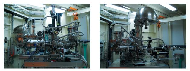
Fig. 5: Photographs of the experimental setup with the electron analyzer oriented horizontally (left) and vertically (right), respectively, thus making use of the geometry dependence of the photoionization cross sections of the different orbitals. (Photon beam is coming from the rear into the chamber, polarization vector horizontal.)
