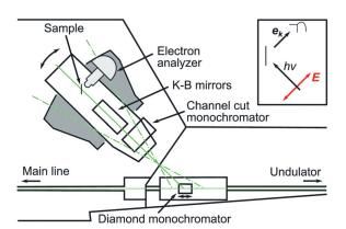
Fig. 4: Top view sketch of the BL12XU (Taiwan Beamline) sideline dedicated to HAXPES at SPring-8. The inset shows the vectors E and  $e_k$  (both in the paper plane) for the *horizontal* setup.
